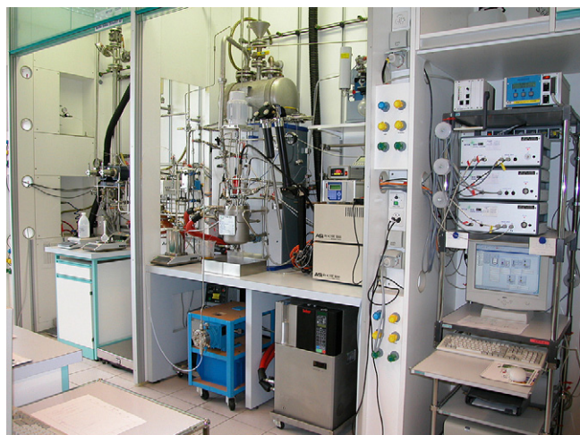
Fig. 6. Typical laboratory system for study of ethynylation reaction parameters.
